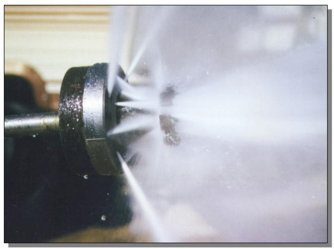
Cleaning head connected to 288 psi (19,8 bar), 48 gpm (182 l/min) water supply.
