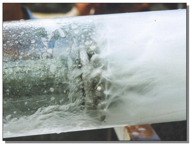
Flow pattern of a cleaning head at 140 psi (9,7 bar) and 160 gpm (606 l/min).
