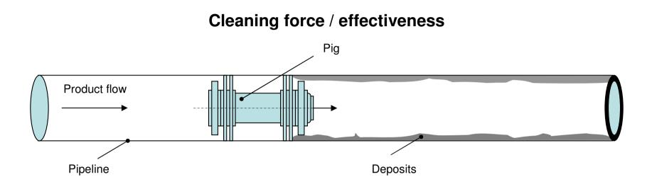
Mechanical force (scraping) between pipe inner wall and the pig's cleaning edge
