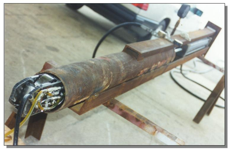
Test set-up to determine the brake systems' travel speed/brake force characteristics. A hydraulic ram was used to pull the brake systems through a pipe section.
