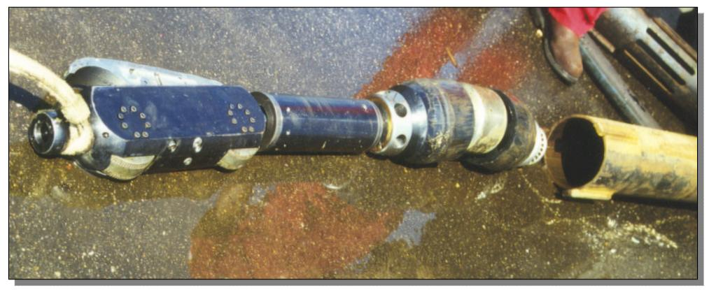
HAPP<sup>™</sup> after a cleaning run of the 7.3 miles, 6.25 inches Braheney Line [operated by Equilon Pipeline Company, Denver City, TX pipeline contained 4 elbows à 22.5°, radius: 1.5 D]
