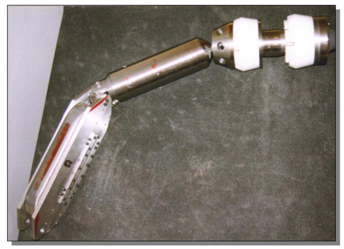
HAPP<sup>™</sup> prototype design based on the cleaning head and brake system tests.
