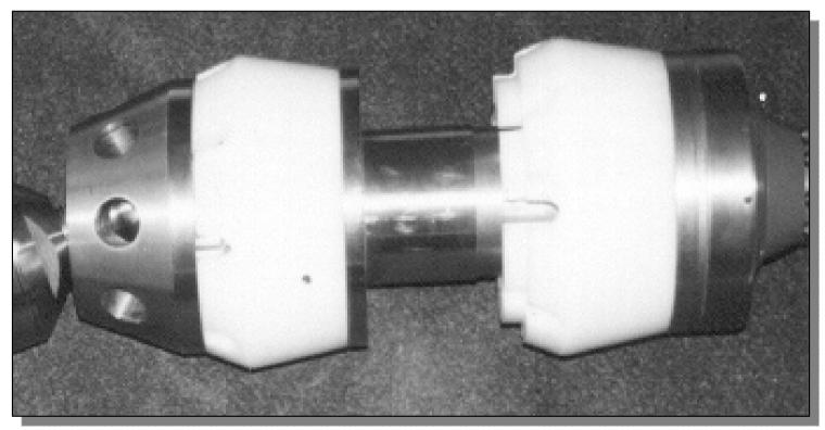
Seal incorporating seal body with polyurethane seal cups.
