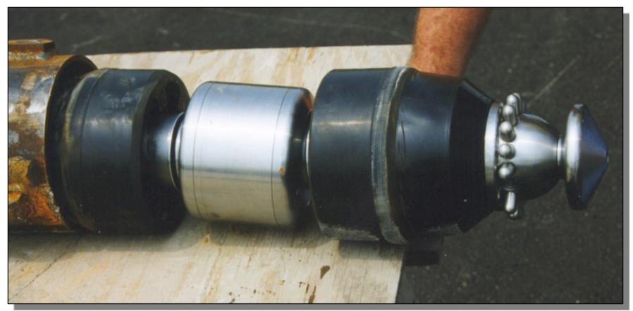
Seal body with rigid and wear resistant seal cups installed.
